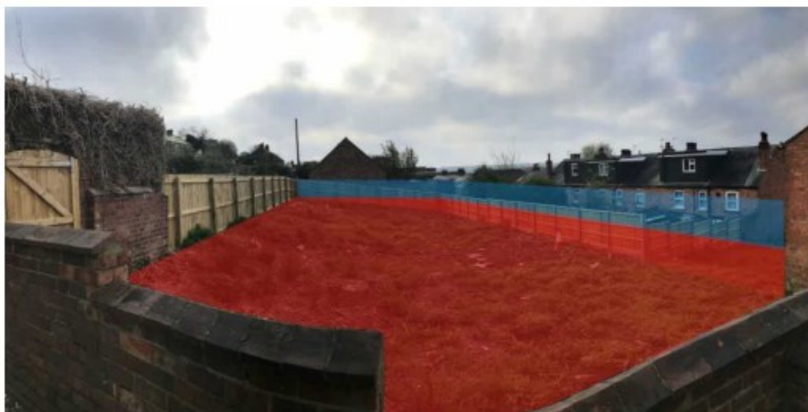
Fig. 11 Illustrating the enormous scale of the proposed terrace earthwork (indicated in red) required to level the site. The proposed boundary fence is indicated in blue. Again,
