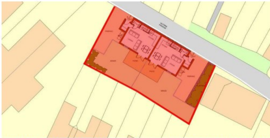
Fig. 10 Scale of the earthwork terrace – the area indicated in red will be new material added onto the hillside to level the site and proximity to properties further down the hill on Victoria Terrace.
